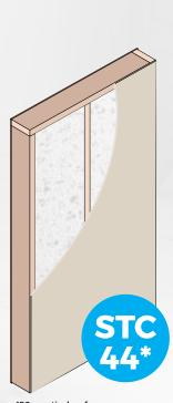
\*90mm timber frame with 10mm plasterboard (two layers on one side)
